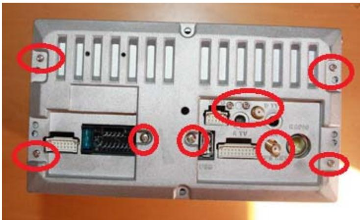
4. Unscrew bottom panel (top panel has sealing).
