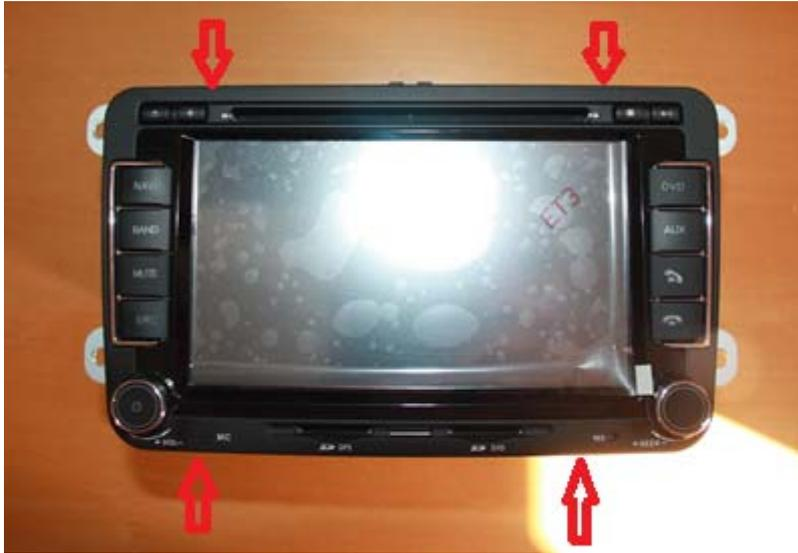
2. Now remove the 4 screws as indicated and remove front metal panel
