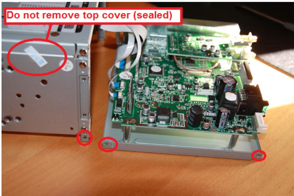
5. Disconnect the 2 flat cables from DVD, now you can Remove also the 4 screws of the PCB
